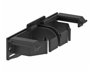
Cover adapter for mounting on trunking bases and fittings of the GAD and Rapid IBIS design device installation trunking series. The cover adapter can be pushed into a guide on the base and is used to accept the trunking cover and keep it at the desired spacing. It is also used for bundled cable exits and can be moved into the lengthwise direction. A maximum spacing of 500 mm between the cover adapters must be maintained.
