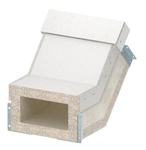
Rising vertical bend for PYROLINE® Con S fire protection duct, type BSKH09-K1021, consisting of fibreglass lightweight concrete which is resistant to water and frost for the creation of vertical changes of direction (45°) of the duct. Mounted connectors ensure quick mounting in situ, whilst loosely placed covers ensure quick inspection and reassignment.
