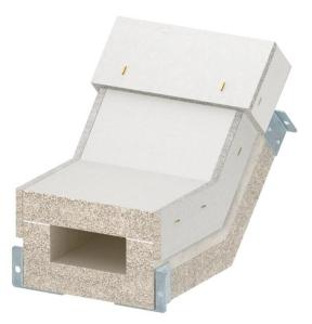
Rising vertical bend for PYROLINE® Con S fire protection duct, BSKH09-K0511, consisting of fibreglass lightweight concrete which is resistant to water and frost for the creation of vertical changes of direction (45°) of the duct. Mounted connectors ensure quick mounting in situ, whilst loosely placed covers ensure quick inspection and reassignment.
