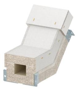
Rising vertical bend for PYROLINE® Con S fire protection duct, type BSKH09-K0506, consisting of fibreglass lightweight concrete which is resistant to water and frost for the creation of vertical changes of direction (45°) of the duct. Mounted connectors ensure quick mounting in situ, whilst loosely placed covers ensure quick inspection and reassignment.
