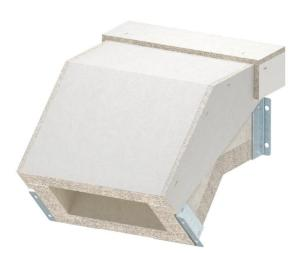
Falling vertical bend for PYROLINE® Con S fire protection duct, type BSKH09-K1021, consisting of fibreglass lightweight concrete which is resistant to water and frost for the creation of vertical changes of direction (45°) of the duct. Mounted connectors ensure quick mounting in situ, whilst loosely placed covers ensure quick inspection and reassignment.
