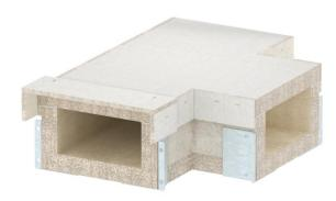
T piece for PYROLINE® Con S fire protection duct, type BSKH09-K1021, consisting of fibreglass lightweight concrete which is resistant to water and frost, for the creation of T branches of the duct. Mounted connectors ensure quick mounting in situ, whilst loosely placed covers ensure quick inspection and reassignment.
