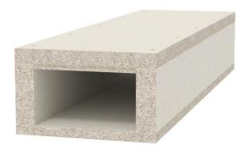
Fire protection duct made from water and frost-proof fibreglass lightweight concrete of building material class A1 according to EN 13501-1 for fireproof laying of cables in rescue and emergency routes, and for the maintenance of electrical functionality of safety-relevant systems. Classification I90 as I duct according to DIN 4102 Part 11 and classification E30 as E duct according to DIN 4102 Part 12.
