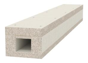
Fire protection duct made from water and frost-proof fibreglass lightweight concrete of building material class A1 according to EN 13501-1 for fireproof laying of cables in rescue and emergency routes, and for the maintenance of electrical functionality of safety-relevant systems. Classification I90 as I duct according to DIN 4102 Part 11 and classification E30 as E duct according to DIN 4102 Part 12.
